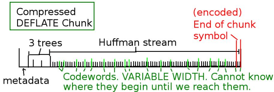
Figure 1: What each chunk looks like. A DEFLATE stream is nothing more than a concatenation of these chunks.
